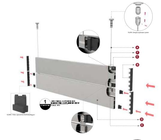
Suspension Sytem "Inox look". Can possibly retaing clip for hanging several profiles one underneath the other.
